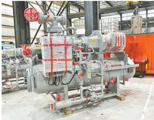
A recently-made compressor, made at the Katy Mayekawa plant, is wrapped and ready for shipment. The company manufactures compressors that serve the food, medical and oil and gas industries.
