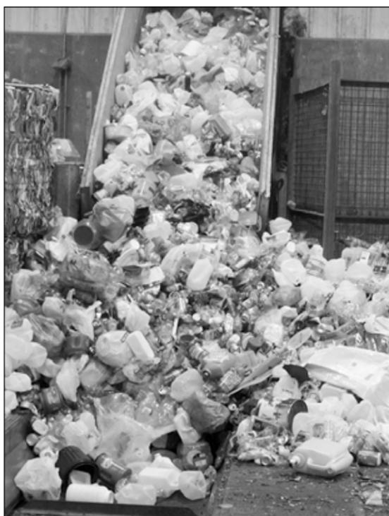
**Recycling ascends a conveyer into the sorting room in Virginia. From here the material is sorted by type before being bailed and hauled away by market buyers. See the sidebar at right for more info on how the county recycling process works.** photo by M. White
