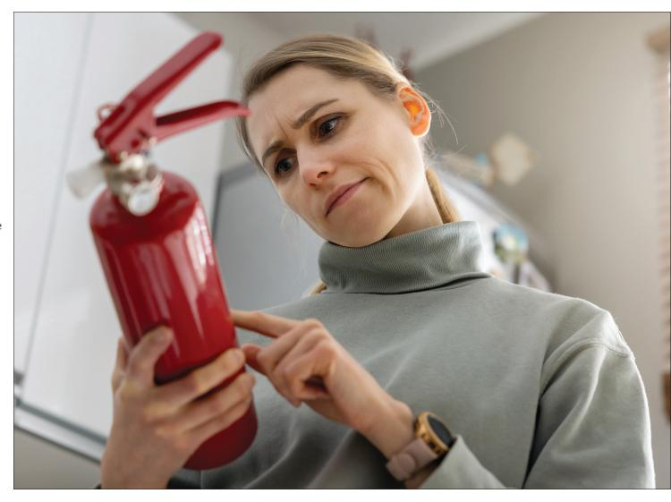
requires maintenance is a fire extinguisher. You can't just buy one and trust it will work forever. Regular inspections ensure its effectiveness. Check the pressure gauge located near the lever of your extinguisher, and look for any visible signs of damage or wear. Most high-quality extinguishers have a lifespan of five to 15 years, but that period can differ depending on the manufacturer.
