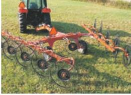
**Hay Rake VR8** The VR hay rake is perfect for changing conditions and uneven terrain with its simple adjustments for windrow and working widths and independent spring suspension, which enables each rake wheel to work individually for a clean sweep. This V-Type rake is available in 8-, 10-, or 12-wheel configurations, and the rake sections fold horizontally over the carriage for narrow transport width and extra stability.
