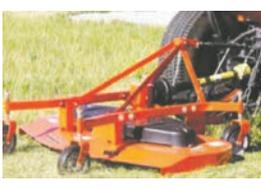
**Finish Mowers** The FA Series Finishing Mower Series features a tapered, sloped discharge area to provide even distribution of cut material across the width of the mower. This allows for less clumping and windrowing than similar mowers that use chain guards or rubber deflectors.
