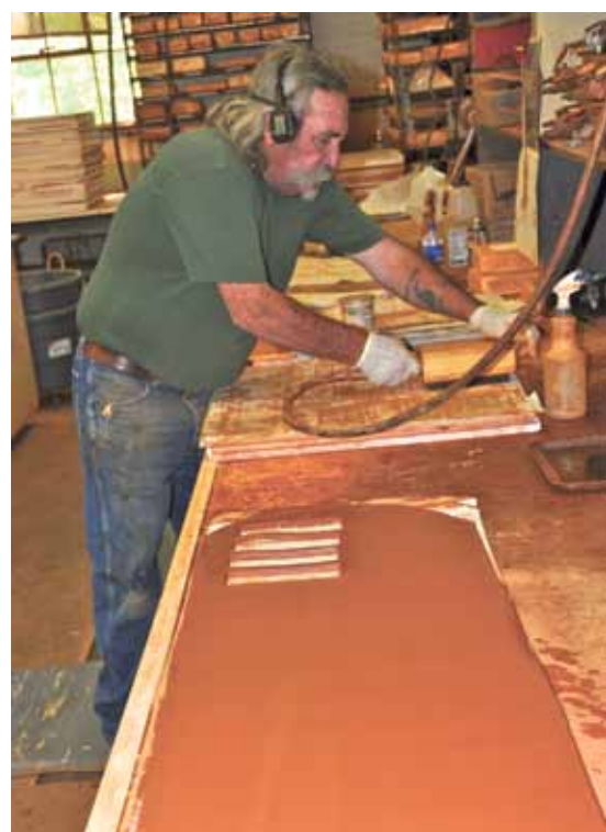
Clay worker Gene Bernier uses a compressed air cutter to cut out each tile by hand.
