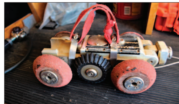
The tiny robotic truck is ready to roll through city sewers, so LCU crews can see any problems and make repairs quickly. That keeps city wastewater flowing smoothly.
