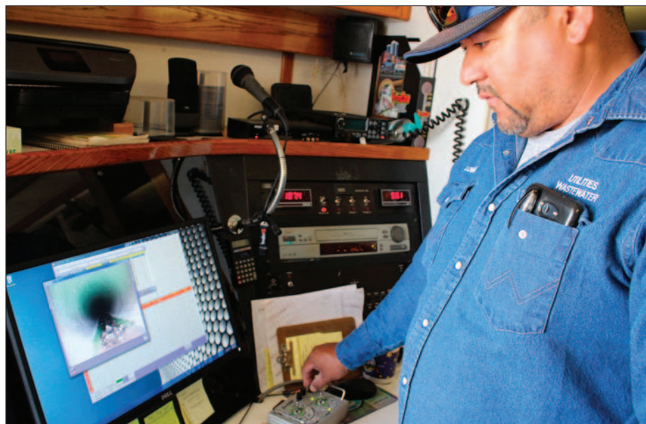
LCU's Lonnie Orona operates the robotic camera that glides through Las Cruces sewer lines to make sure the pipes are healthy. Technology like this helps LCU "see" in areas too small for crews to go.
