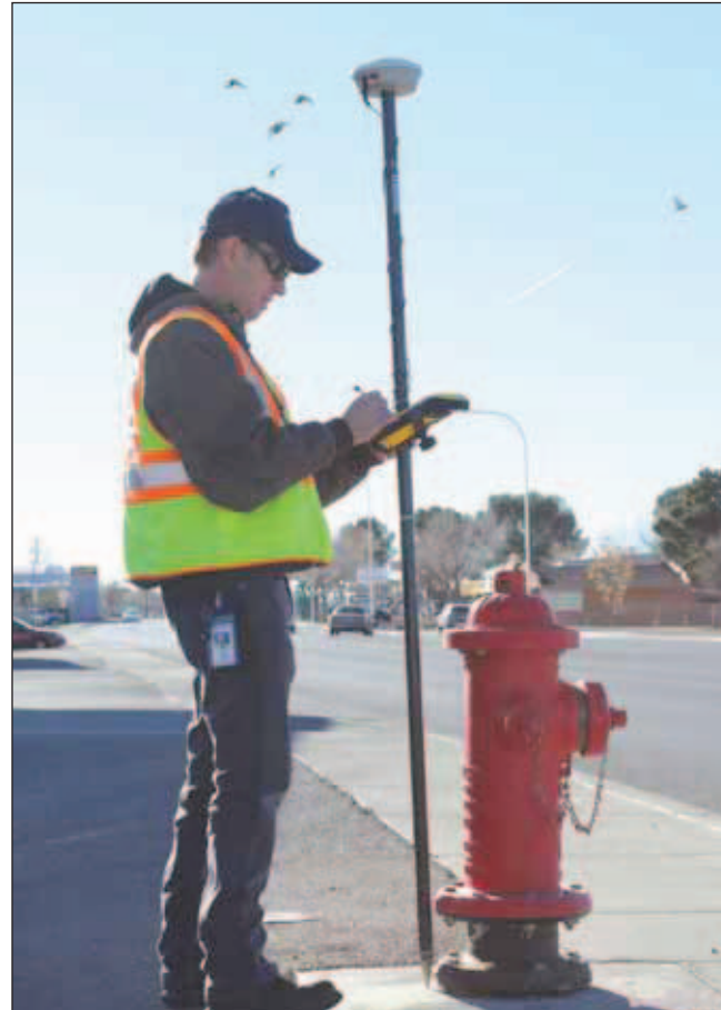
Matt Anderson, graphic information system analyst, uses a GPS data collector to input the exact location of a fire hydrant on North Valley Drive.
