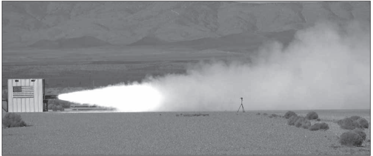
SpaceLoft Rocket Motor Qualification Static Test conducted Oct. 9 at Spaceport America.
