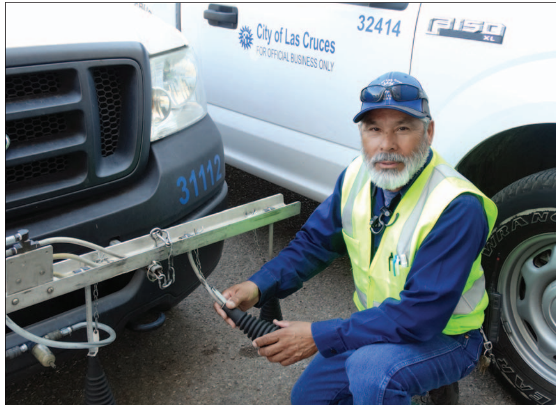
Adam Valles, leak survey technician, shows one of the cones mounted on the front of the LCU leak survey trucks. The cones suction in and test the air immediately above the street pavement.
