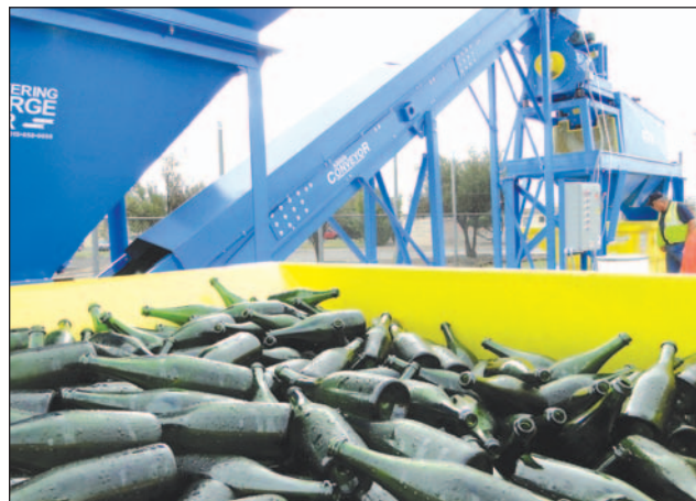
Green wine bottles are loaded into the SCSWA's industrial-sized glass crusher.
