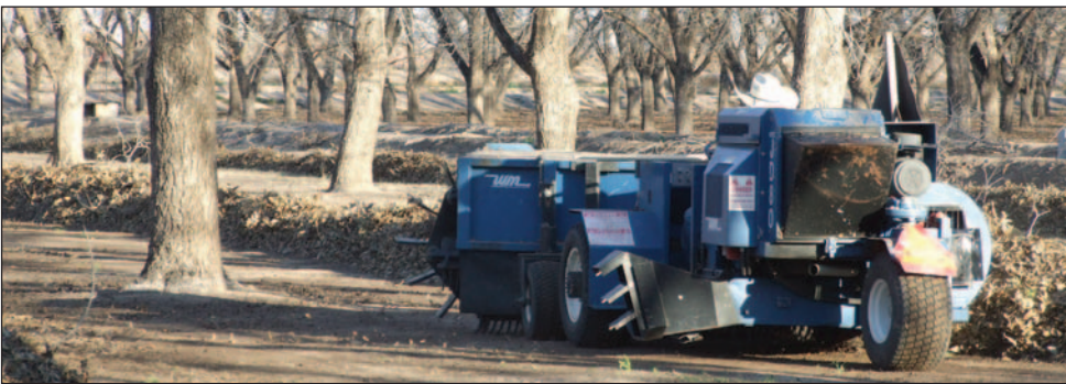
After trees were shaken with a boom, Pasco Jimenez sweeps pecans and leaves into piles for transport to the processing facility.
