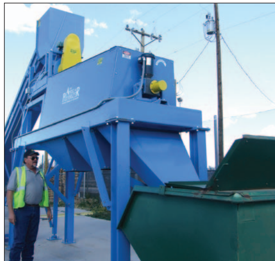
The crusher can process three or four tons of glass at a time. Each load is crushed in about an hour.
