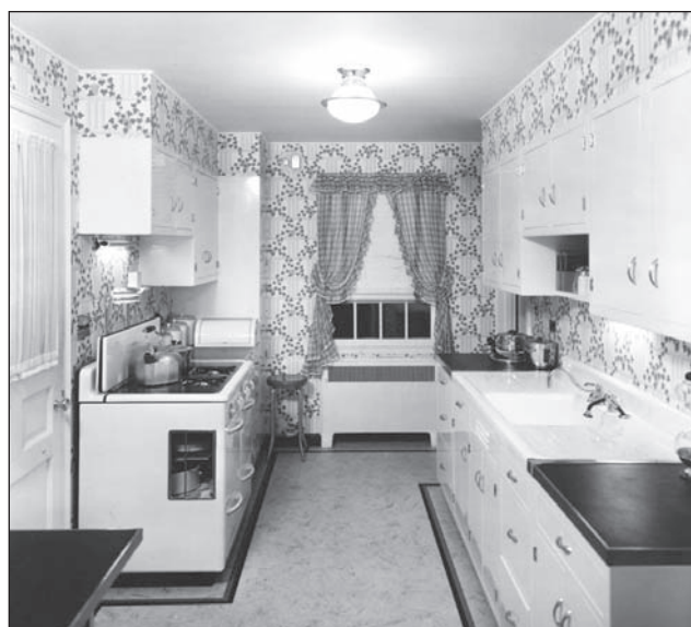
The Kitchen of Tomorrow, as it appeared at the 1939 New York World's Fair, demonstrated the latest trends in kitchen design, including built-in cabinets and continuous counter space.
