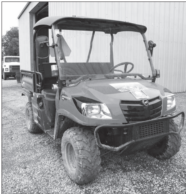
One of two ATVs used on campus and powered by biodiesel fuel made from waste cottonseed oil discarded after being used in restaurant fryers.
