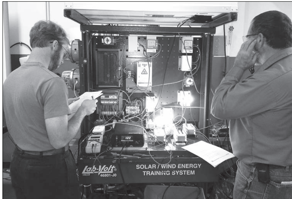
Students Kris Harig and Michael Knowles in the PV Power Generation Design Fundamentals class at New Mexico State University-Alamogordo assemble the circuitry for installing a photovoltaic (solar) system. They are working on a Lab Volt trainer.
