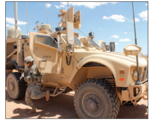
SPC Allison Miracle, who supports communications for the brigade commander, steps out of a vehicle part of the Warfighter Information Network-Tactical (WIN-T), which provides mobile satellite connectivity to Brigade Commanders. WIN-T is a system under test in NIE 13.2
