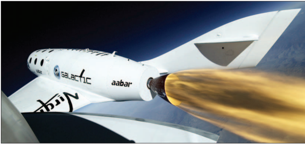
View of SpaceShipTwo's rocket motor and plume during the 16-second burn Monday, April 29, as seen from the spaceliner's burn camera.
