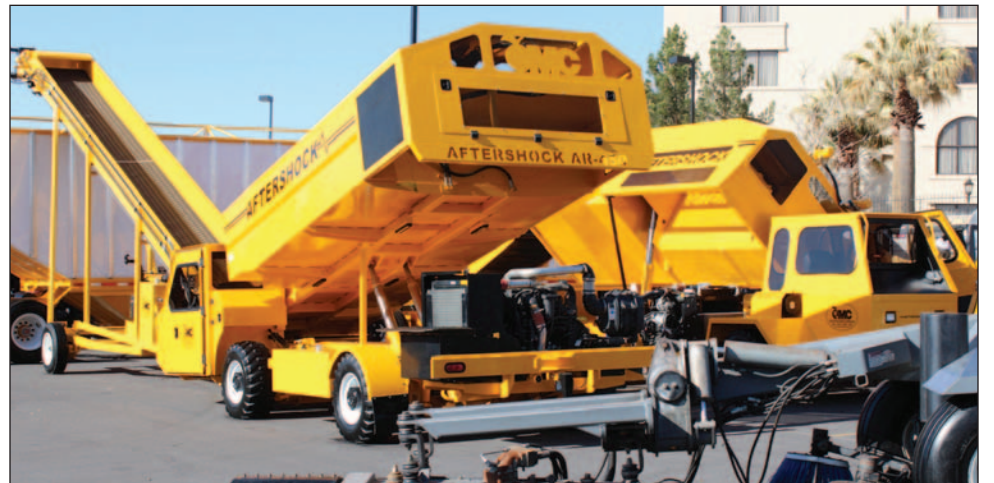
The Aftershock AR450 is a machine that gets filled with the pecans and transfers them to a field elevator processor or the pecan processing plant.
