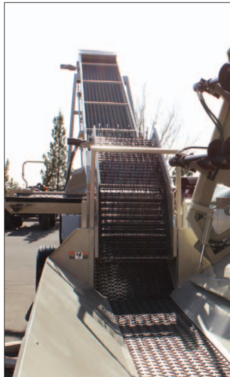
The pecan field elevator processor used for large pecan orchards.
