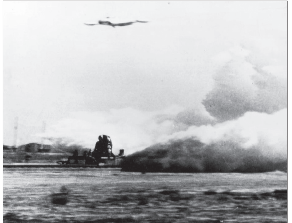
U.S. Air Force/New Mexico Museum of Space History Archives The water-braking system that brought Dr. John Stapp to an abrupt halt plumes spray behind him. Piloting the chase plane above him is Capt. Joe Kittinger.
