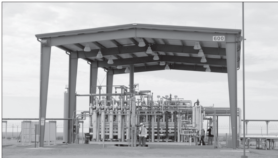
Concentrated algae is processed through these units, where it becomes "green crude" oil at the Sapphire Energy Las Cruces Test and Development Site at the West Mesa Industrial Park.
