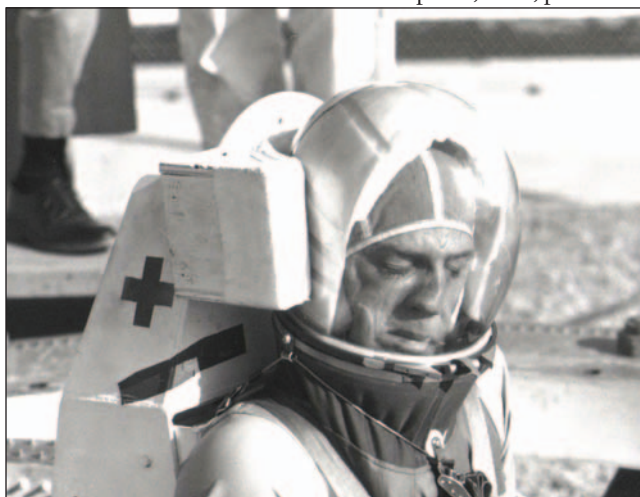
This is a close-up of a test subject's face as it is distorted during sudden deceleration.
