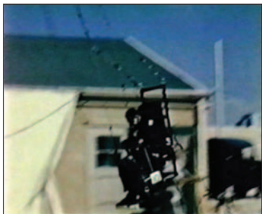
These United State Air Force images are from a film taken in September 1956, showing Dr. John Paul Stapp during a Swing Seat test that gauged the effectiveness of seat belts. A cable pulled Stapp back, and at release he swung forward until the cable jerked him – painfully – to a stop.
