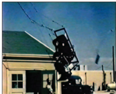
These United State Air Force images are from a film taken in September 1956, showing Dr. John Paul Stapp during a Swing Seat test that gauged the effectiveness of seat belts. A cable pulled Stapp back, and at release he swung forward until the cable jerked him – painfully – to a stop.
