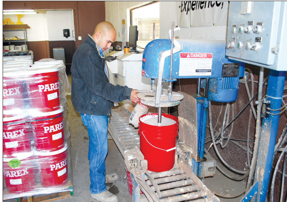
Las Cruces Bulletin photo by Beth Sitzler Josh Hernandez, L & P Building Supply and Components' go-to "tint and color guy," waters a mixing batch of custom-colored stucco at the company's facility.
