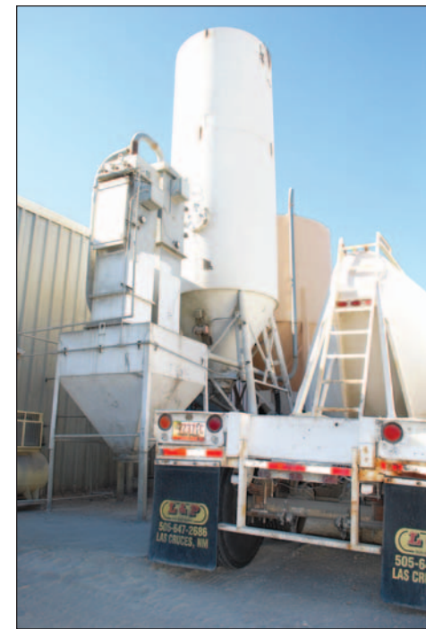
The company also has its own silo to mix and bag concrete products.
