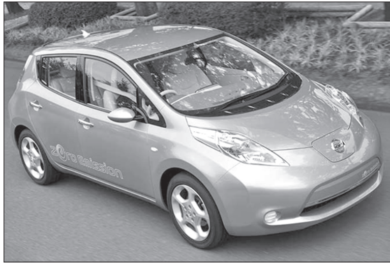
Most electric cars, such as the Nissan Leaf, have a battery charge that will last 100 to 130 miles.
