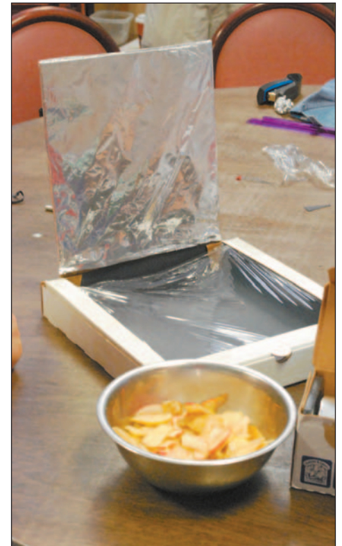
When completed, the pizza box solar ovens can be used to cook fruits, vegetables and even already-made cookie dough in a few hours.
