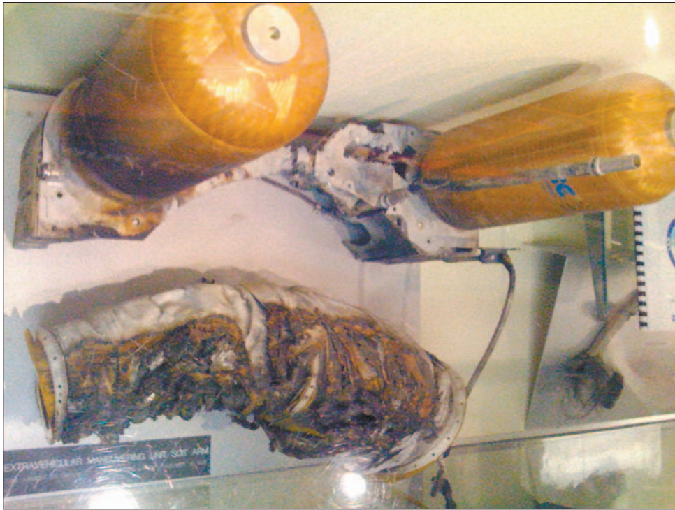
This display case at the NASA White Sands Test Facility in Las Cruces shows two oxygen tanks and an extravehicular maneuvering unit suit arm that were damaged by leaking oxygen as part of test exercises performed by Jacobs Technology.
