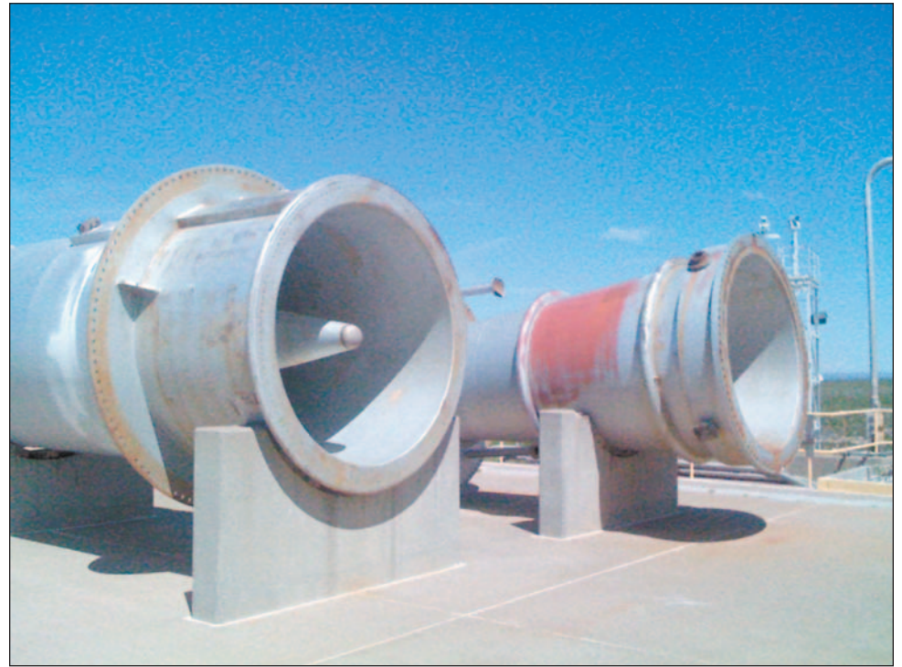
These rocket test chambers located at the NASA White Sands Test Facility are part of Jacob Technology's Jet Propulsion Systems test area.
