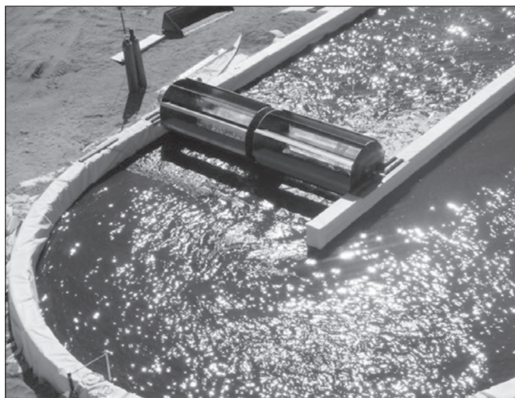
This machine churns the water to keep it constantly moving in an algae pond at the West Mesa Sapphire Energy research center.
