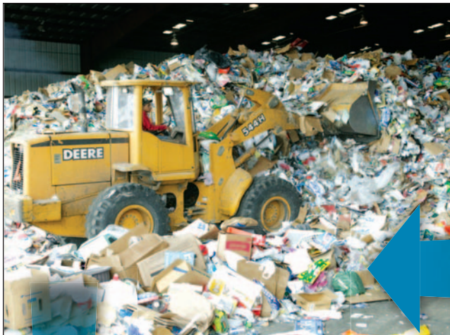
The aluminum can is mixed with all other recyclables brought from Las Cruces and emptied onto the "tripping floor," where front-end loaders place them on fast-moving conveyor belts.
