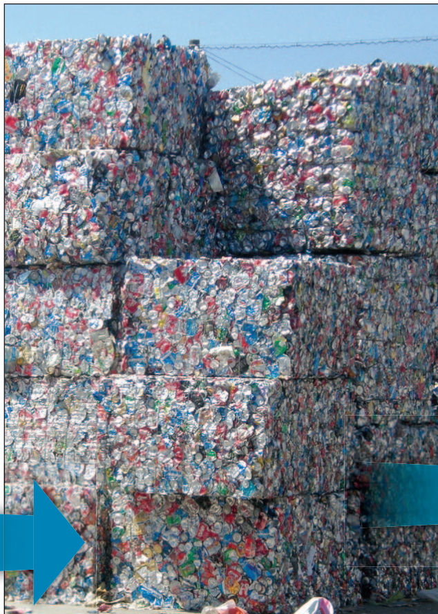
Aluminum cans are baled and shipped around the country to be transformed into new products. At Friedman Recycling, 80 to 100 bales – weighing 1,500 to 1,800 pounds each – are recycled daily.
