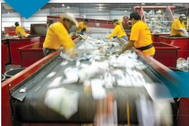
The recyclables are then pre-sorted by hand by six employees, and the aluminum can is placed with other cans.
