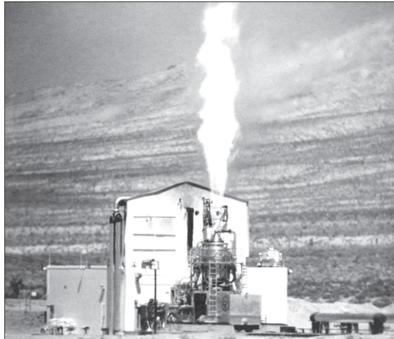
The Kiwi-A test nuclear rocket engine test, on June 20, 1959, was the first for Project Rover. Afterward, a remotely controlled miniature train engine pushed the “hot” engine, at one mile an hour, to a safe area for examination.
