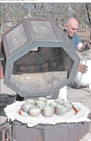
The kiln Mott uses heats to 500 degrees, was built from steel and uses propane to heat.
