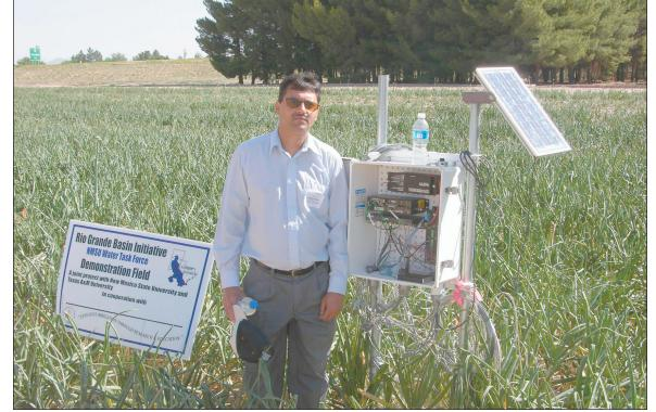
NMSU assistant professor Manoj Shukla explains how the solar-powered field sensor measures and records soil salinity, moisture content and temperatures during Onion Field Day at the university.
