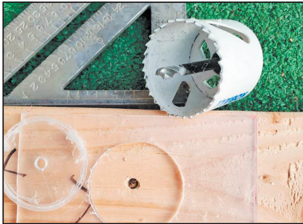
Creating arm holes in the COVIDBox prototype with a saw made by NMSU students.
