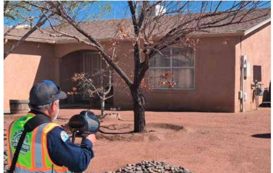
LCU Gas Leak Surveyor Adam Valles aims his RMLD at a gas meter. The detector can work from the street and gives Valles an exact percentage of the leak if he finds one.
