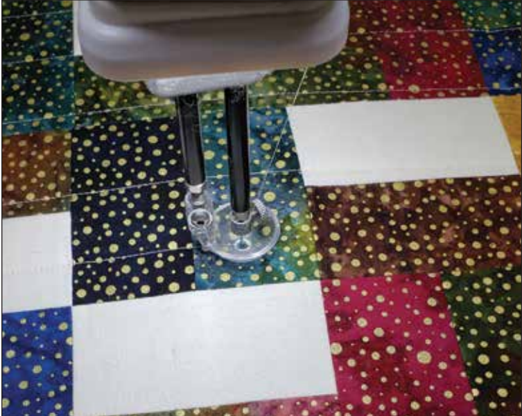
Quilting straight lines on the longarm quilting machine. (Photos by Mia Kalish)
