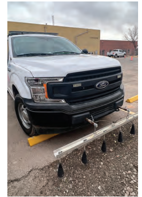
LCU leak survey truck - Courtesy LCU
