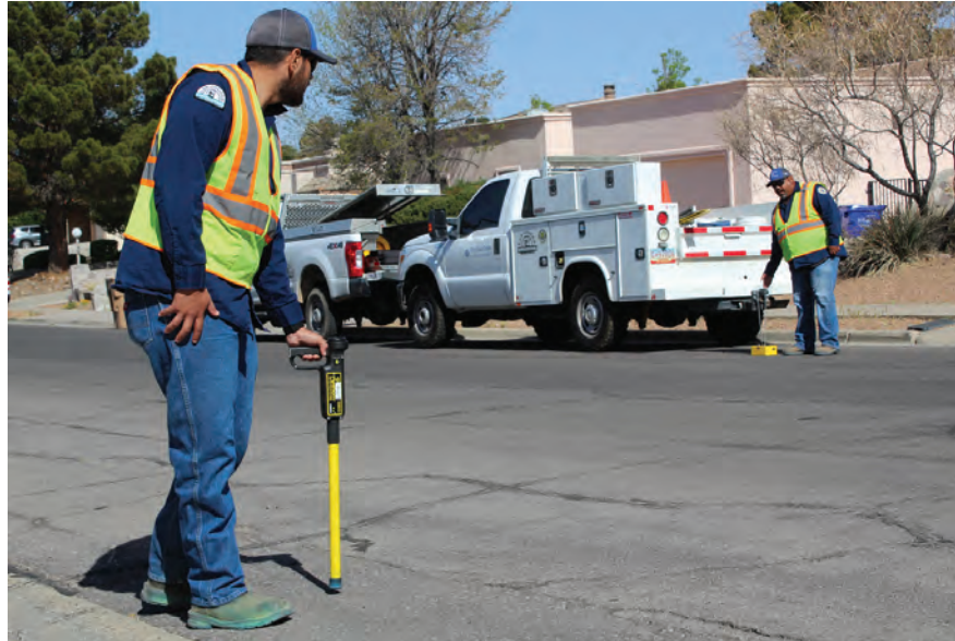
Utility Line Locators George Pallares and Benjamin Garcia in the field using inductive locating with a transmitter and receiving in older neighborhoods where pipes lack tracing wires that are now on all installed pipes in the system.
