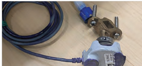
Leak Sensor - Courtesy LCU
