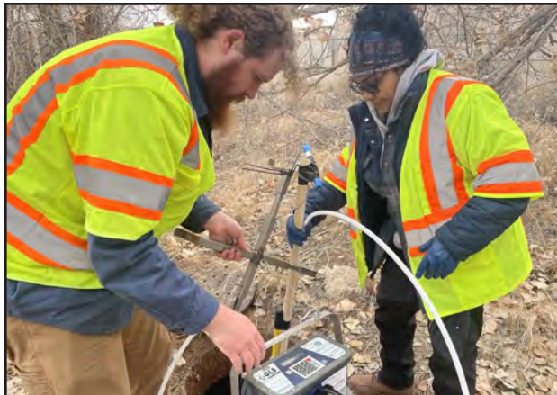
COURTESY PHOTO BY KUNM NEWS Tom Brown, an employee with Eastern Research Group, lowers tubes into a sewer behind Belen High School to test the wastewater.
