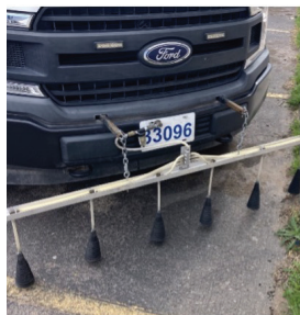
A natural gas infrared detector mounted to the front bumper of an LCU Leak Surveying vehicle
