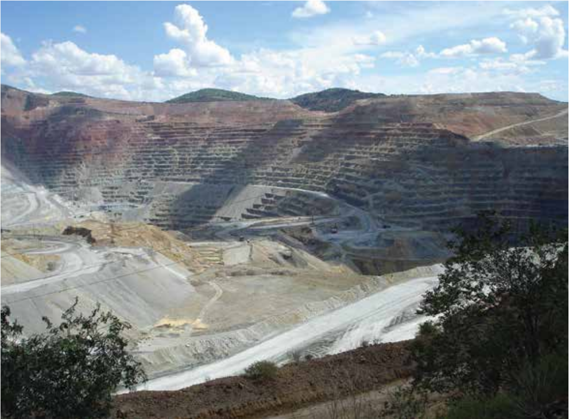
Terraced wall of Chino Mine pit is where ore is extracted.
