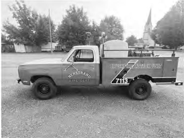
4 Wheel Drive 8 cylinder 360 CID, Automatic Transmission, Odometer states 16,487 but actual Miles unknown. Comes with a 200 gal tank, 23hp pump, and hose reel with 100' of booster line.
