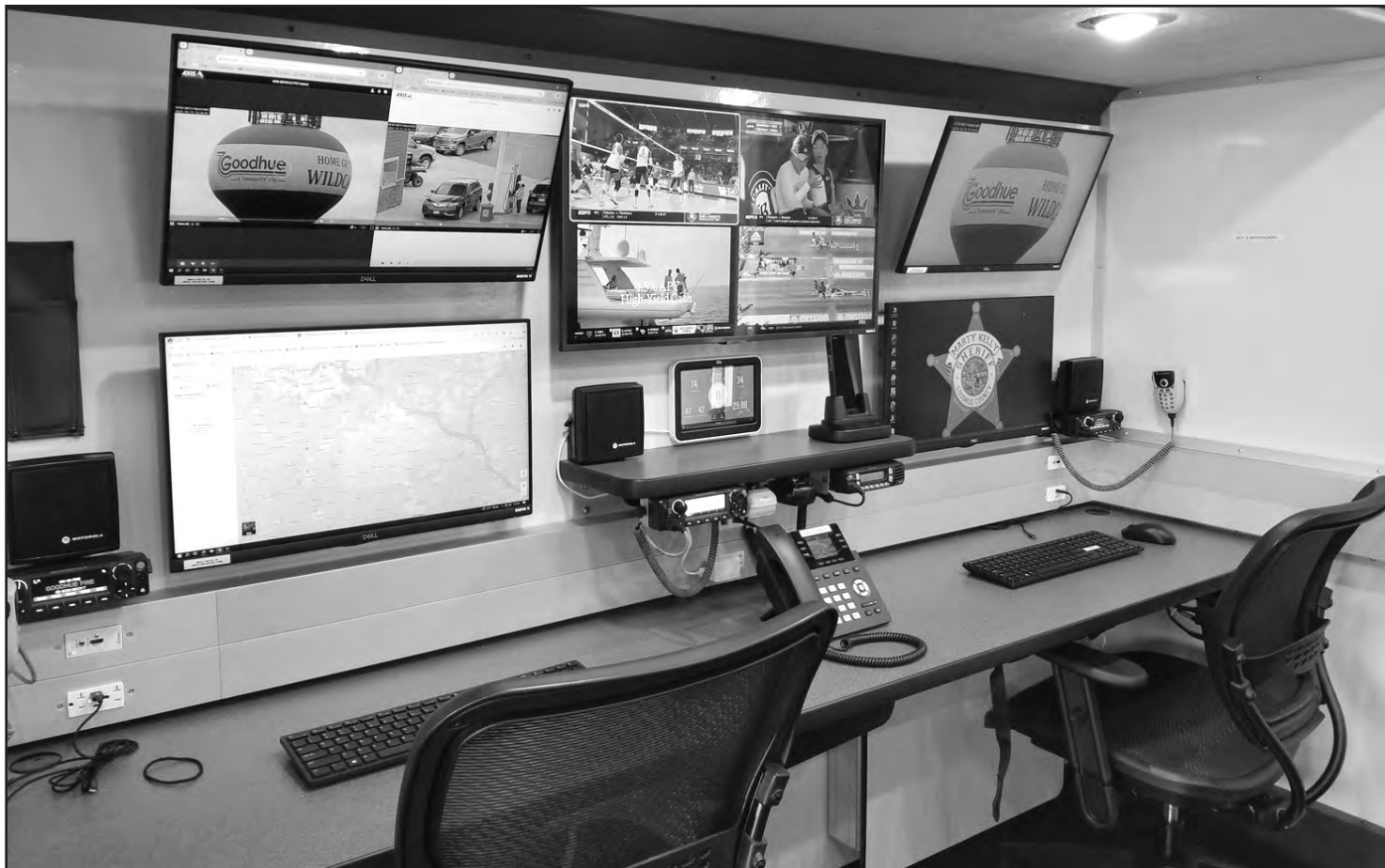
The mobile command unit is capable of doing everything that can be done at the main office including taking 911 calls and sounding alarms. It can be separated into sound-proof areas where officers can monitor screens connected to cameras both along the unit's perimeter and on a mast with a 1-mile range.
