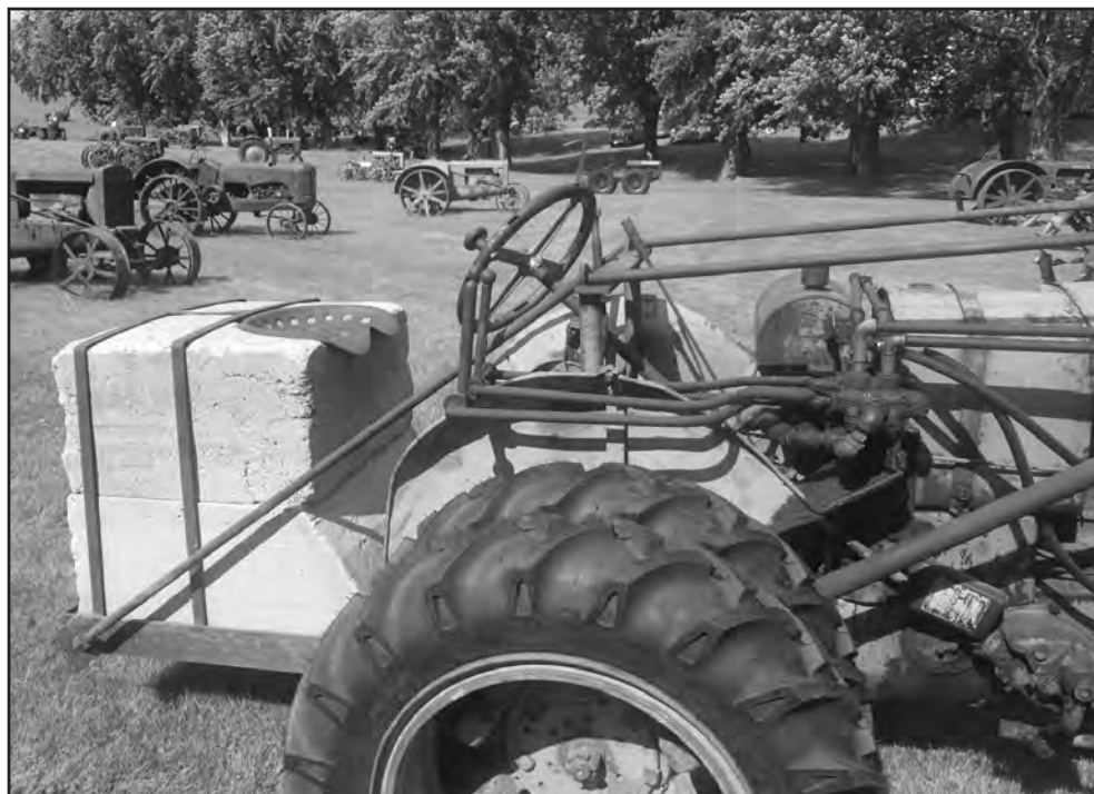
The weight may counter a load on the front bucket of this tractor, but does not provide the most comfortable seating.
