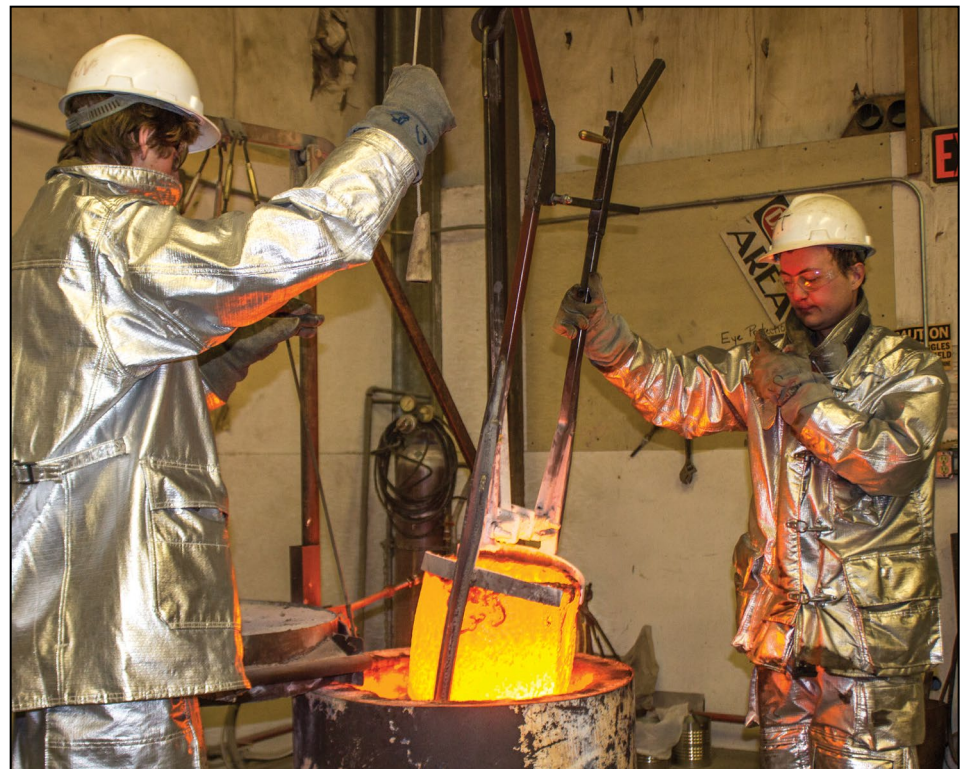
Above and Below and at Right: Jessie Thomas, lead foreman in molding and melting, right, carefully navigates a vat of molten metal out of a 3,000 degree furnace, pouring it into various molds.
