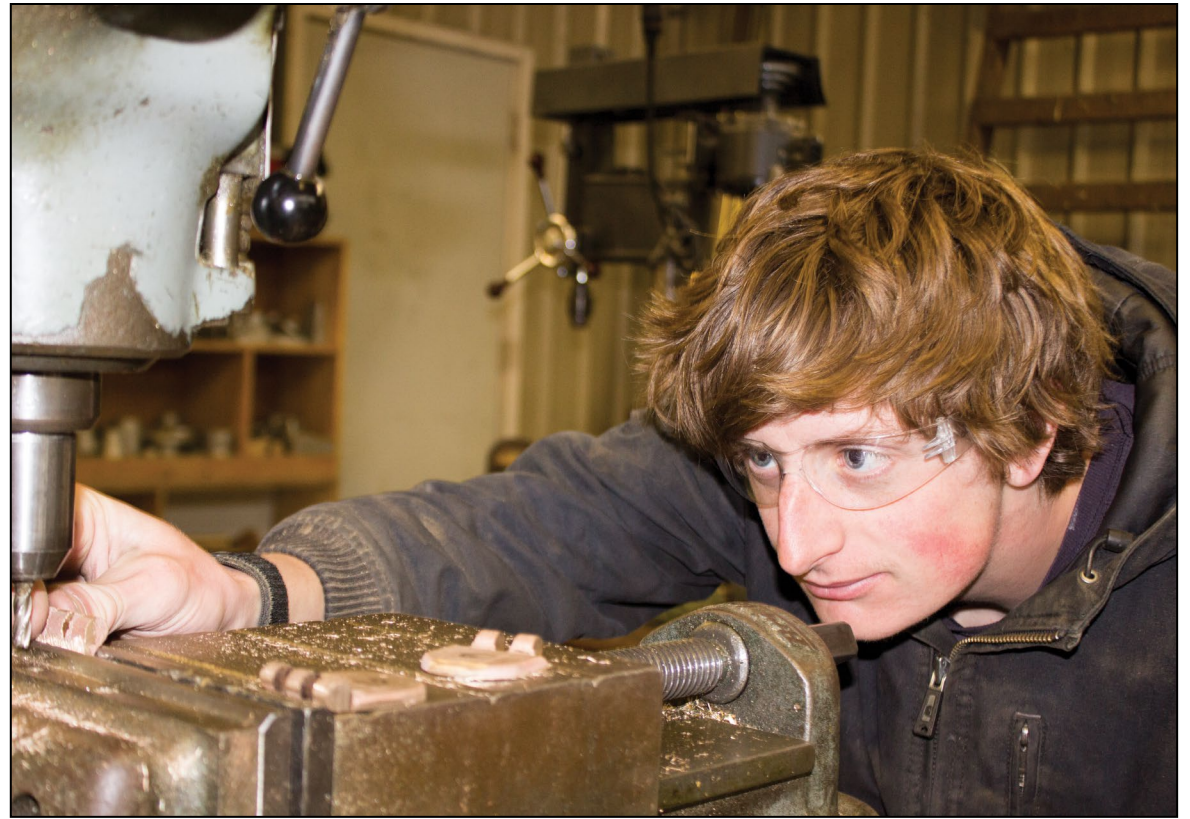
Daniel Burgess, machinist, cleans up the slots of bronze hinges so they fit together nicely. The hinges will be used on hatches or cabinetry on a boat that will participate in the 2019 Race 2 Alaska. They do not rust and will last a century if properly maintained. Leader photos by Chris McDaniel
