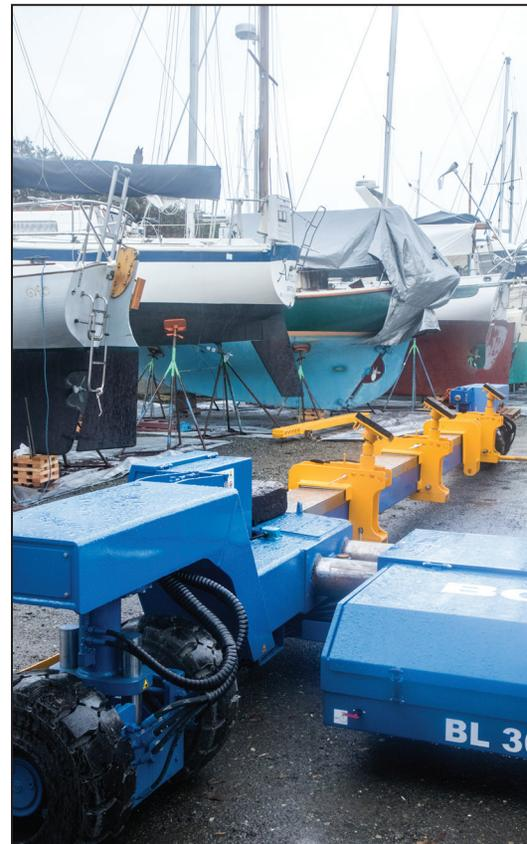
The trailer is operated by remote control, and the operator can extend the size to fit different boats.
