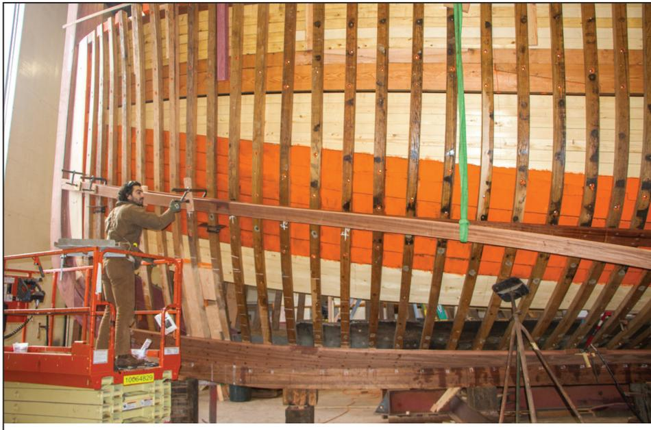
Shipwright Ryan Bard clamps a first plank in place where it cools into the complex shape of the hull from stem to stern.
