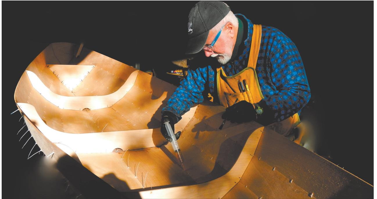
Marty Loken works to assemble a small wooden boat using stitch-and-glue construction. Photo courtesy Marty Loken
