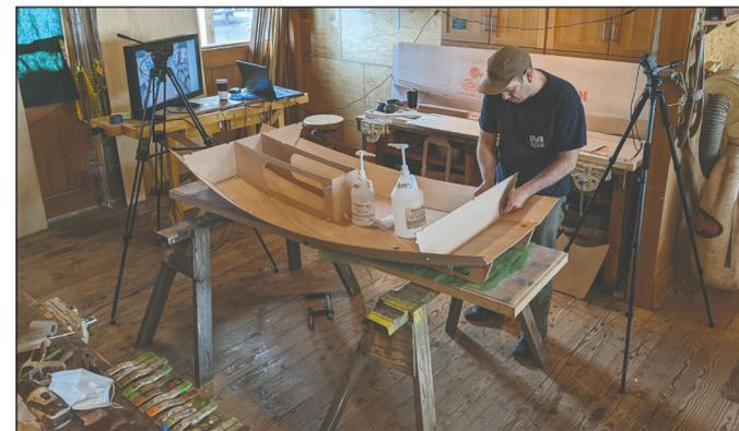
Liam Crist-Dwyer assembles a small boat called a “Portage Pram” using the glue-and-stitch construction method. Photo courtesy of Northwest Maritime Center
