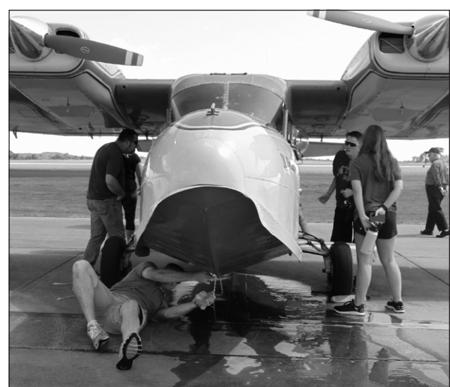
The pilot of this sea plane had to pump water that collects in the bilges after landing on water.
