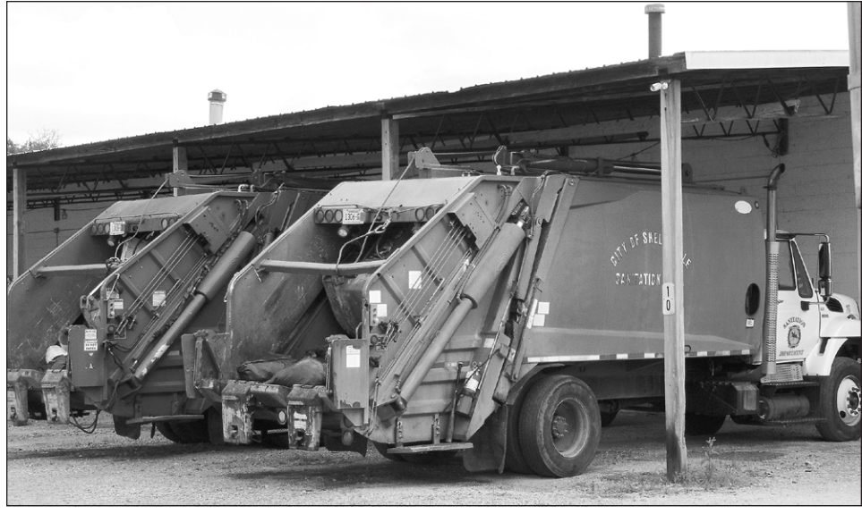
These rear-loader garbage trucks require two men working in the back. Public works director Buck Vallad said they hope to purchase two more side-arm automated trucks which require only one driver and make route management more efficient.
