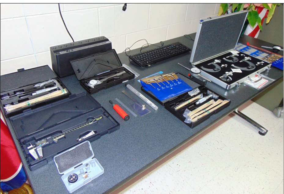
With the Gordon Scholarship award, recipients get to purchase tools of the trade, such as micrometer gauges, calipers, scribes, and burrs pictured here.
