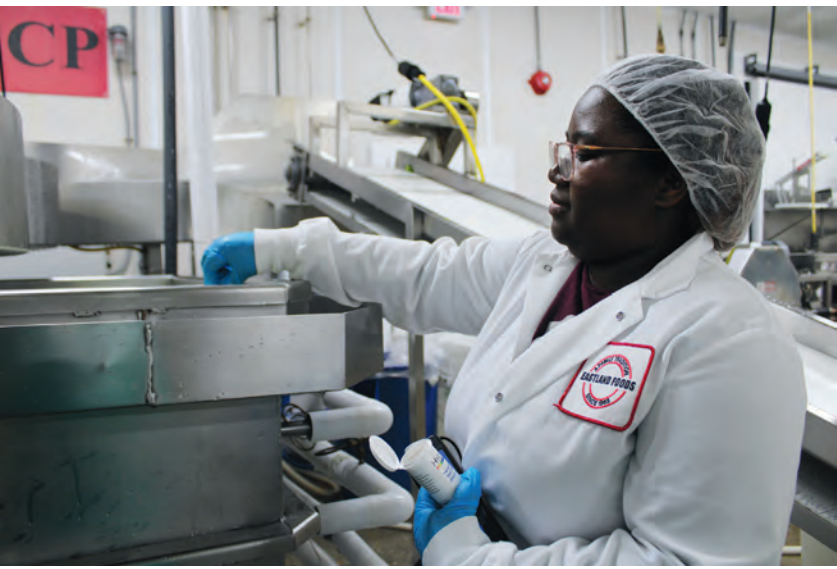
QUALITY CONTROL: QA Manager Diva Gomes tests the concentration of peracetic acid in the water on the onion processing line. The test comes back positively, with the concentration level within the acceptable range.
